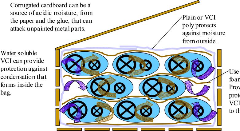
Use VCI paper or foam as a separator. Provides mechanical protection and the VCI has free access to the metal
